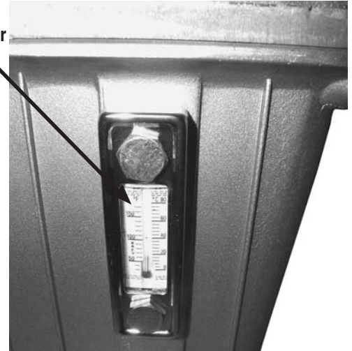
Oil Level And Temperature Meter
